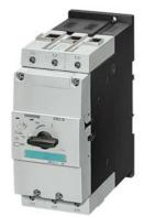
Circuit breaker size S3 for motor protection, Class 10 A-release 45...63 A Shortcircuit release 819 A Screw terminal Standard switching capacity !!! Phased-out product !!! Successor is SIRIUS 3RV2 Preferred successor type is >>3RV2031-4JA10<<
